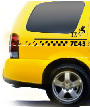
TLC Smart Design Logo side decal placement; black ink, located near rear window. [source: TLC website]
